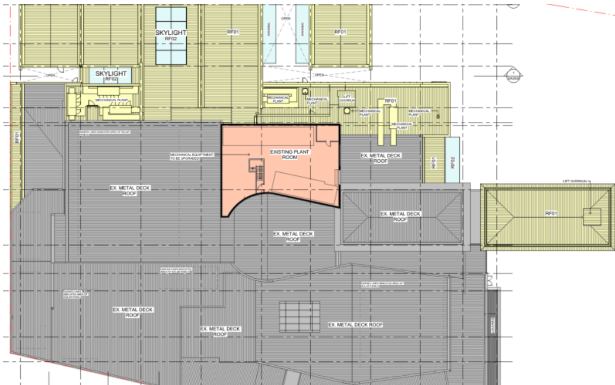
Figure 1: Level 2 plant room only contains plant and therefore is not counted in the rise in storeys as per C2D3(2)(a). New roof area in yellow is the new Porte Cochere connecting from the club building to the new car park building.
